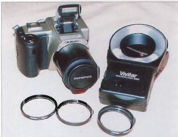
Fig. 2: The Olympus C2500L digital camera is an example of the megapixel cameras that may be used for clinical photography. The single-lens reflex system and through-the-lens focusing of these cameras make them very similar to the 35-mm cameras with which most of us are experienced. After-market ring flash and macrolenses are available.
