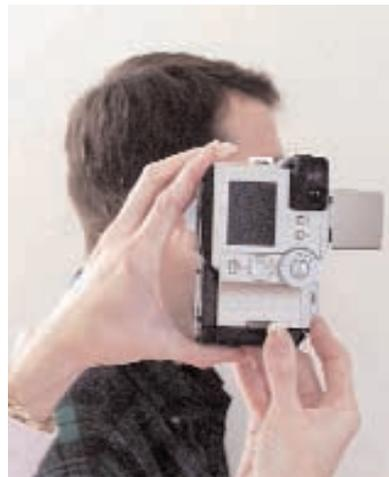
**Figure 27.2** The problem of a flash attachment being mounted too far away from the lens is illustrated; the closer the flash is to the lens, the better suited the camera is to macrophotography.
