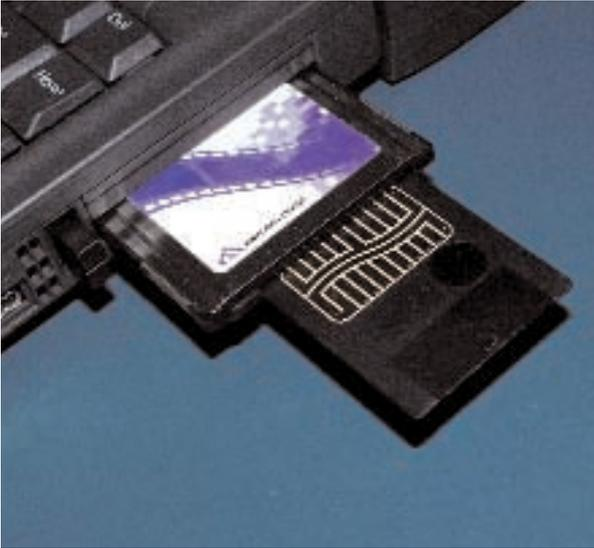
*Figure 27.5* PCMCIA card-readers are available for the SmartMedia storage cards. The SmartMedia card simply inserts into the PCMCIA card which, in turn, inserts into the computer.
